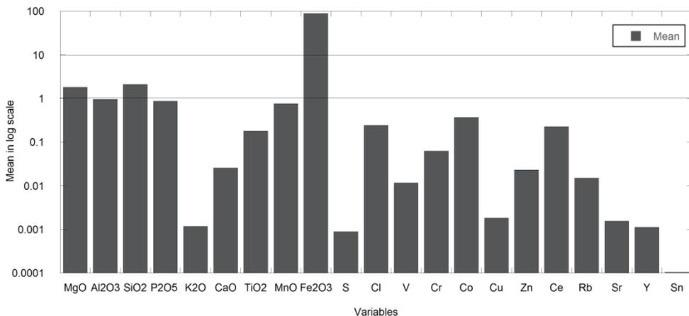
Figure 2. Measured mean XRF data in logarithm scale.
