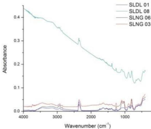
Figure 1. Analysed FTIR graphs of the limonite samples using Origin labfor SLDL 01, SLDL 08, SLNG 03, and SLNG 06
